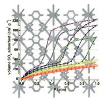
MOFs on the move: A new, twofold interpenetrated metal–organic framework (MOF) material has been synthesized that demonstrates dramatic steps in the adsorption and hysteresis in the desorption of CO<sub>2</sub>. Powder X-ray diffraction measurements and pair distribution function analysis indicate that structural changes upon CO<sub>2</sub> sorption most likely involve the interpenetrated frameworks moving with respect to each other.
