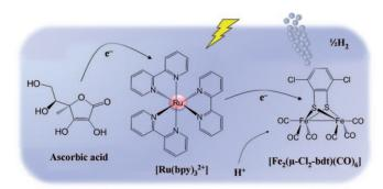
**Lifting the diiron curtain**: 200 equivalents of  $H_2$  per catalyst at a maximum turnover rate of 3.7  $H_2$  per minute can be obtained in a light-driven proton
