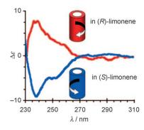
Majority-rules effect: We report a strong majority-rules effect in the formation of chiral dynamic nanotubes from chiral bisurea monomers. The same helical nanotubes can be obtained from racemic monomers in a chiral solvent (see figure). Competition experiments revealed the relative strength of the helical bias induced by the chiral monomer or by the chiral solvent.
