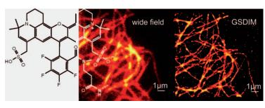
Optical nanoscopy labels: New rhodamine dyes and their reactive derivatives are proposed as efficient photostable fluorescent labels for imaging in the red optical region, which is very important for biological studies (see picture). The dyes feature high fluores-
